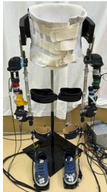
Fig.2 MALO: Motor Actuated Lower-limb Orthosis
