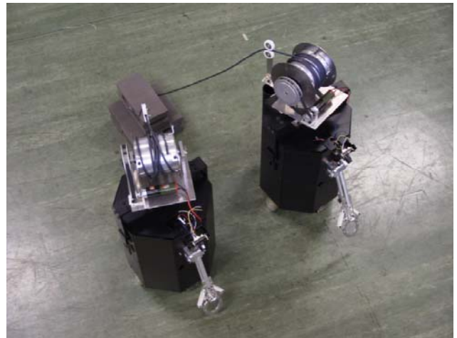
Figure 13 The mobile robots tugging an object with tethers
